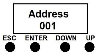
Use UP and DOWN to scroll through the available choices. Push ENTER when you reach the option you want to check or set. The current setting for the option will be shown. Use UP and DOWN until you reach the desired setting or menu then push ENTER to invoke the new setting. Use ESC to exit from the sub menus.
