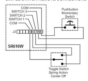
The example uses a Lightronics APP01 switch station and a momentary pushbutton switch. If the SR616W simple switch functions are set to factory default operation the switches will operate as follows.
