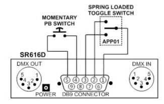
If the SR616D simple switch functions are set to factory default operation the switches will operate as follows for the connection example shown above.
