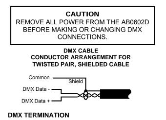
A DMX bus should be terminated (only) at the last receiving device on the chain. This is done by connecting a 120 ohm, 1/4 watt resistor across the DMX DATA - and DMX DATA + lines.
