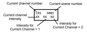
Use the  $\uparrow$  and  $\downarrow$  buttons to set the channel output intensity. The display shows the intensity setting as a number between 0% and 99%. A 100% setting is indicated by "FL". A "XX" setting means that the channel will be ignored for the current scene. This is useful when stacking of scenes is desired.
