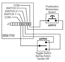
If the SR617W simple switch functions are set to factory default operation, the switches will operate as follows.
